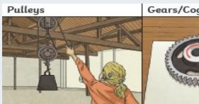
Pulleys can be used to make a small force lift a heavier load. The more wheels in a pulley, the less force is needed to pull the weight.
