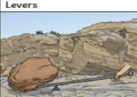
Levers can be used to make a small force lift a heavier load. A lever always rests on a pivot.
